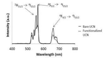
Figure 3. The upconversion emission spectra, under 980 nm excitation of bare and functionalized UCN Y<sub>2</sub>O<sub>3</sub>:Er<sup>3+</sup>/Yb<sup>3+</sup> (1%, 1% mol) green emission (564 nm) in <sup>4</sup>S<sub>3/2</sub>→<sup>4</sup>I<sub>15/2</sub> transition is present.
