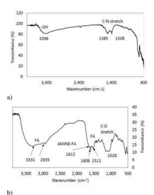
Figure 4. FTIR spectra of a) bare UCN  $Y_2O_3$ :Er<sup>3+</sup>/Yb<sup>3+</sup> (1%,1% mol) and b) functionalized UCN-NH<sub>2</sub>-FA.
