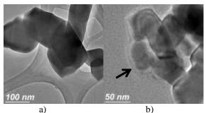
**Figure 2.** TEM images of UCN  $Y_2O_3$ :  $Er^{3+}/Yb^{3+}a$ ) bare and b) functionalized UCN-NH<sub>2</sub>-FA. The black arrow indicates the silica-coating.
