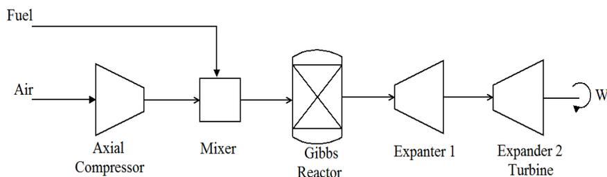
Figure 4. Flow diagram of a gas turbine.
