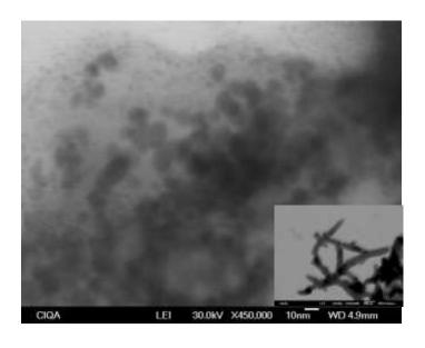
**Figure 3**. STEM micrographs of magnetic nanoparticles embedded into PANI-FFe<sub>3</sub>O<sub>4</sub> nanocomposite and nanocomposite fibres (inset).
