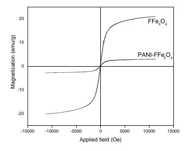
Figure 1. Magnetization curves of a) magnetic fluid and b) PANI-FFe<sub>3</sub>O<sub>4</sub> nanocomposite.
