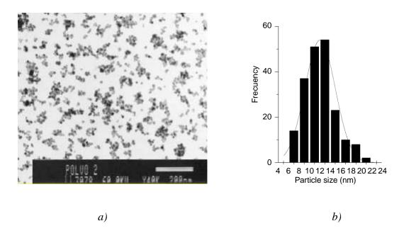
**Figure 2.** a) Photograph of TEM of magnetite obtained by coprecipitation method, and b) particle size distribution of magnetic particles.
