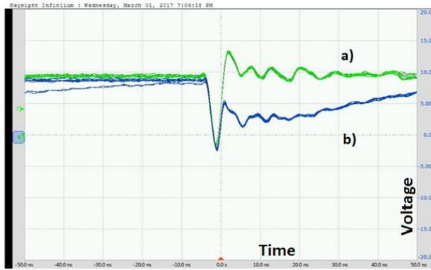
**Figure 9.** Signals obtained experimentally with the LED drive: a) Q2 commutation signal, b) Cathode falling voltage.
