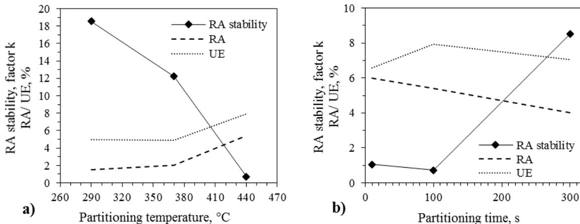
**Figure 12.** Retained austenite stability factor: a) as a function of partitioning temperature (PT) of specimens partitioned for 100s and b) as a function of partitioning time (Pt) for specimens partitioned at 440 °C. Smaller  $k$  values indicate higher stabilization of retained austenite. RA: retained austenite, UE: uniform elongation.
