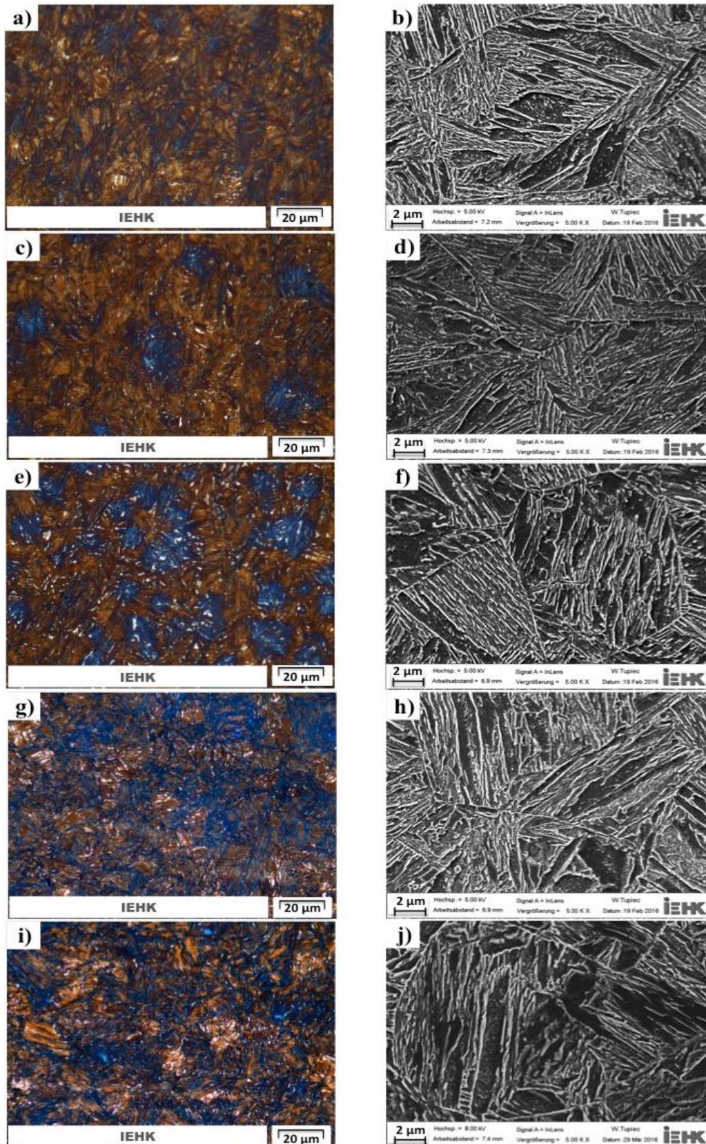
**Figure 6.** Klemm etched LOM micrographs (on the left) and Nital etched SEM micrographs (on the right) for Q&P specimens: a, b) 290 °C-100s, c, d) 370 °C-100s, e, f) 440 °C-100s, g, h) 440 °C-10s, and i, j) 440 °C-300s.
