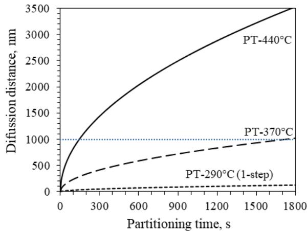
**Figure 11.** Diffusion of carbon in austenite as a function of time for partitioning at 290 (1-step), 370 and 440 °C.
