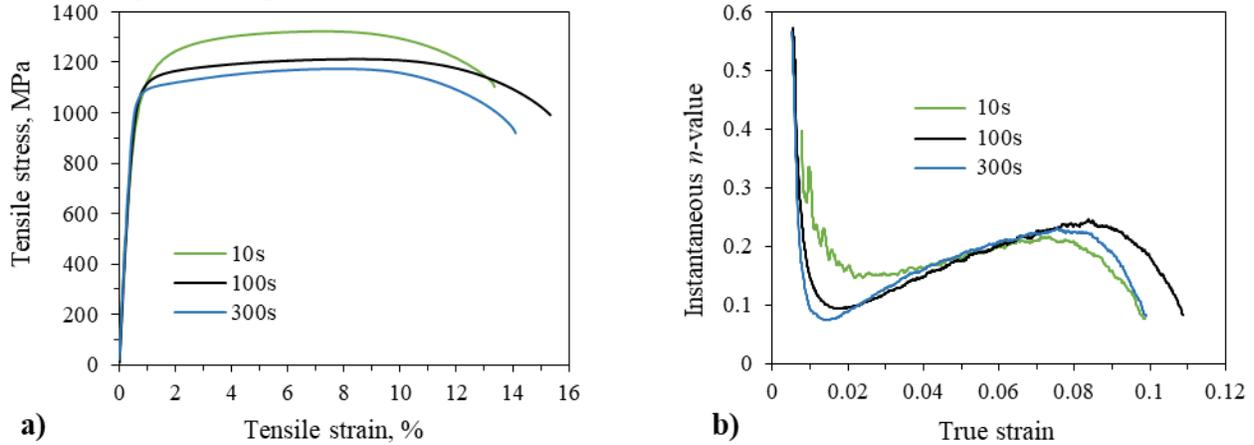
**Figure 9.** Plots of a) engineering stress-strain curves and b) instantaneous  $n$ -value versus true strain for specimens partitioned at 440 °C for 10, 100 and 300s.
