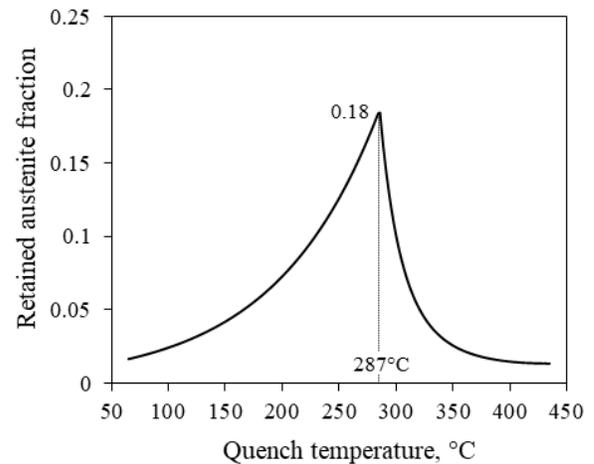
**Figure 1.** Calculated volume fractions of retained austenite as a function of the quenching temperature for the studied CSiMn steel.
