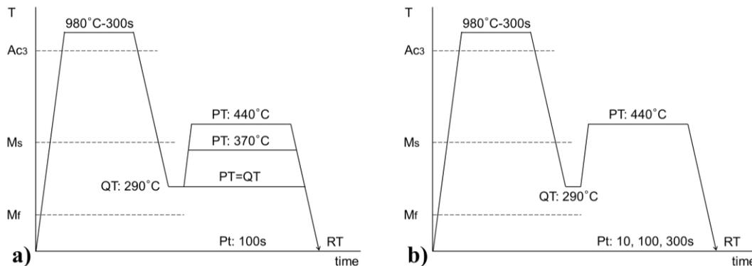
**Figure 2.** Scheme of the Q&P treatments applied to the CSiMn steel to a) evaluate the effect of partitioning temperature (PT) and b) to evaluate the effect of partitioning time (Pt).
