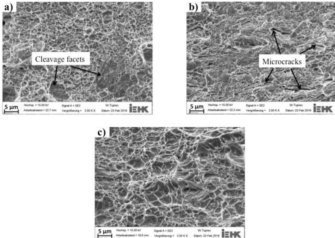
**Figure 7.** Fracture surface of tensile specimens partitioned at: a) 290 (1-step), b) 370 and c) 440 °C for 100s.
