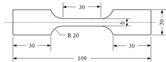
**Figure 3.** Geometry of the tensile specimen. Dimensions are given in mm.
