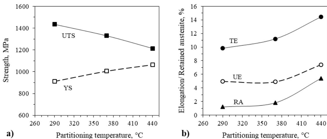
**Figure 4.** a) Tensile properties and b) elongation and retained austenite for specimens partitioned at 290 (1-step), 370 and 440 °C for 100s. UTS: ultimate tensile strength, YS: yield strength, TE: total elongation, UE: uniform elongation, RA: retained austenite.
