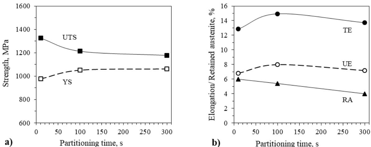
**Figure 5.** a) Tensile properties and b) elongation and retained austenite for specimens partitioned at 440 °C for 10, 100 and 300s. UTS: ultimate tensile strength, YS: yield strength, TE: total elongation, UE: uniform elongation, RA: retained austenite.
