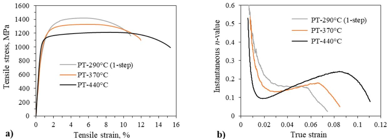
**Figure 8.** Plots of a) engineering stress-strain curves and b) instantaneous  $n$ -value versus true strain for specimens partitioned at 290 (1-step), 370 and 440 °C for 100s.
