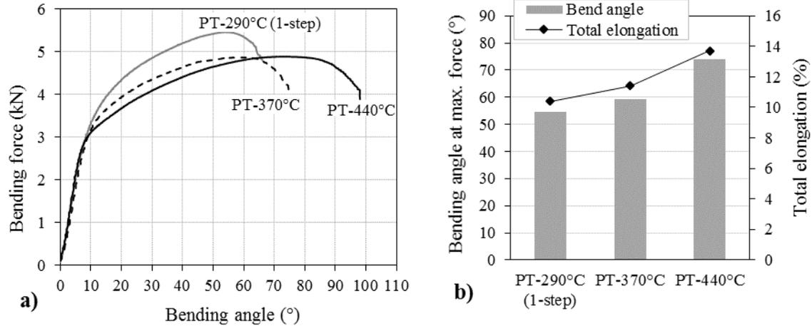
**Figure 10.** a) Bending force/angle curves and b) bending angle at maximum force and total elongation for specimens partitioned at 290 (1-step), 370 and 440 °C for 100s.
