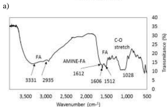
a) b) **Figure 4.** FTIR spectra of a) bare UCN  $Y_2O_3:Er^{3+}/Yb^{3+}$  (1%, 1% mol) and b) functionalized UCN- $NH_2$ -FA.
