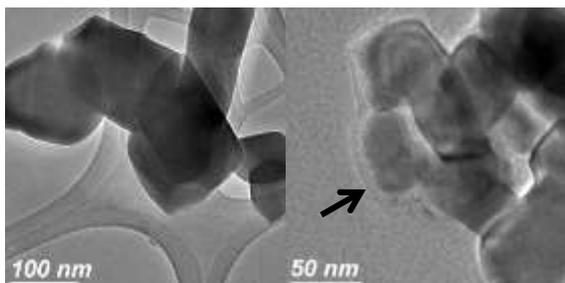
a) b) **Figure 2.** TEM images of UCN  $Y_2O_3: Er^{3+}/Yb^{3+}$  a) bare and b) functionalized UCN- $NH_2$ -FA. The black arrow indicates the silica-coating.
