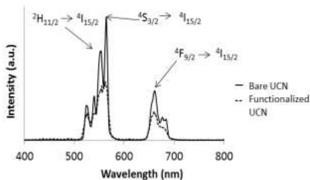
**Figure 3.** The upconversion emission spectra, under 980 nm excitation of bare and functionalized UCN  $Y_2O_3:Er^{3+}/Yb^{3+}$  (1%, 1% mol) green emission (564 nm) in  $^4S_{3/2} \rightarrow ^4I_{15/2}$  transition is present.
