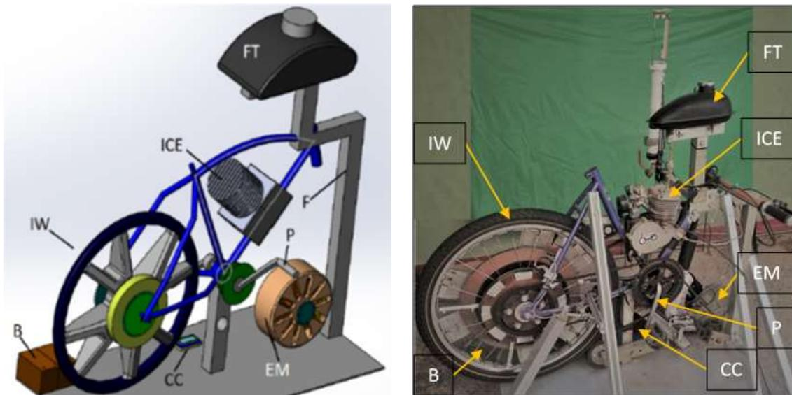
**Figure 1.** The general layout of the devices consists of a stand that supports a bicycle frame (F) that holds the fuel tank (FT), combustion engine (ICE), electric motor (EM), inertia wheel (IW), pedals (P), batteries (B) electronics and control circuit (CC).
