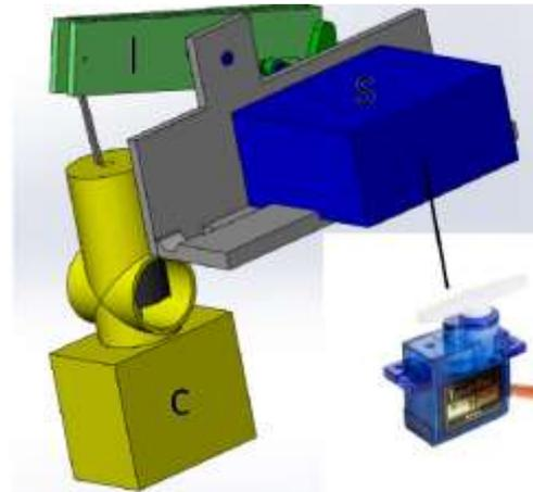
**Figure 7.** Electro-mechanical device to control the A/F mixture. It consists of a servo motor (S) coupled to a lever (L). At the other end of the lever, there is the throttle cable that operates the carburetor (C).
