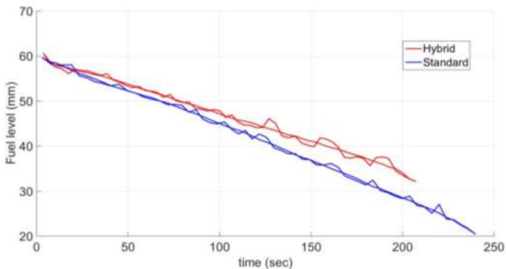
**Figure 11.** The figure shows the fuel consumption as a function of time with and without the use of the DCEM. The straight lines are moving averages showing the fuel saving rate for the hybrid case.
