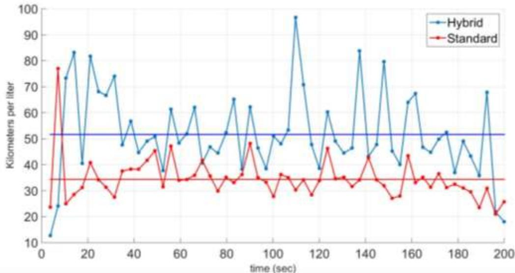
**Figure 12.** The graph is a time series of the kilometers per liter achieved with and without the aid of the DCEM. The flat lines are the average of each run.
