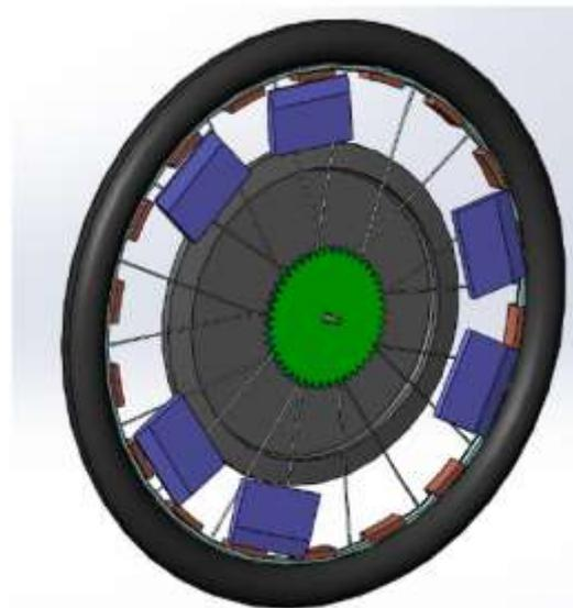
**Figure 3.** The load consists of the original wheel whose moment of inertia has been increased using a concentric weight plate and masses at the edge of the rim. The render shows only one gear of the multiple gear set.
